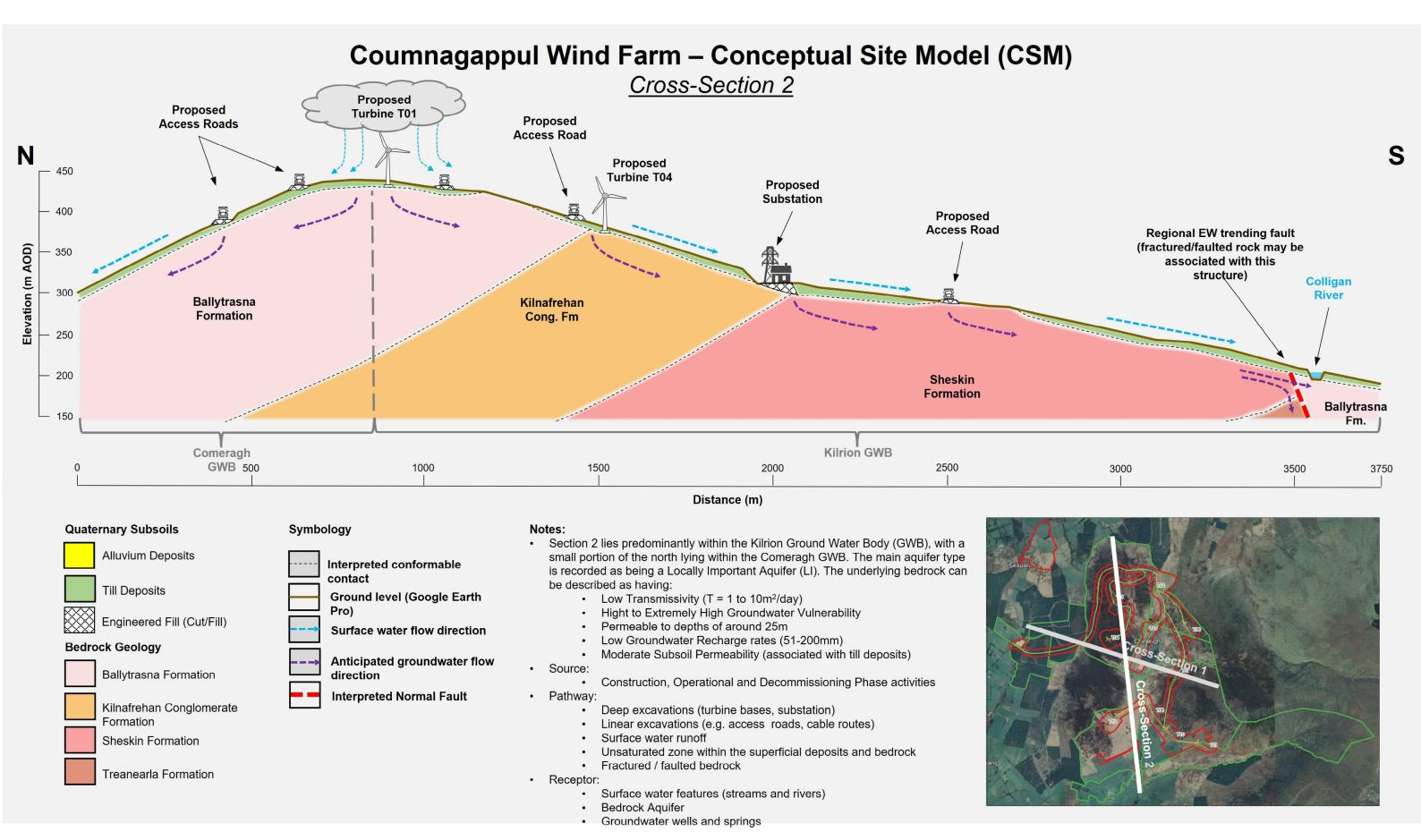
Figure 11.4: Conceptual Site Model (CSM) – N-S Cross-Section
